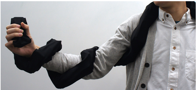
Figure 9. LineFORM wrapped around an arm to constrain body motion.
