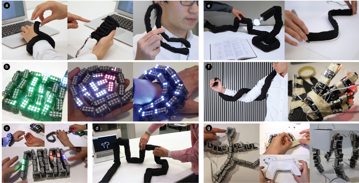
Figure 5. Potential applications on actuated line-based interfaces (a: mobile device, b: display, c: modular display, d: CAD modeling tool, e: ruler and cable, f: body augmentation, g: prototyping tool)
